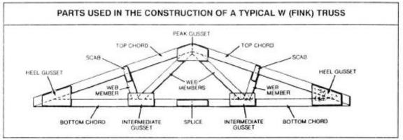
A truss is made up of top chords, bottom chords, and web members tied to the chords with gusset plates. Gussets shown in this drawing are made of plywood.
