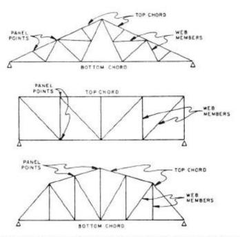
Three basic types of trusses. There are many designs for trusses, each with its own name.
